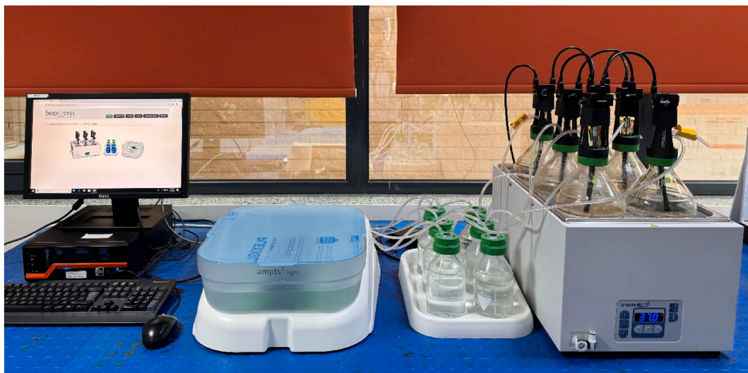
Fig. 1. AMPTS II setup for batch experiments, including the sample incubation unit, CO 2 absorption unit, and gas volume measurement unit connected to a computer for live monitoring.
